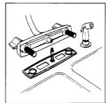
3 Position putty plate. Apply Teflon tape to spray outlet on body. Attach spray hose to spray outlet by rotating faucet body. Tighten securely with wrench.
